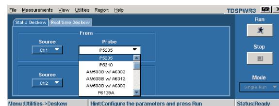
9. Push the "Running Man" button to start taking measurements. If the measurement is successful, the application automatically displays the results. You can also view the results by selecting View> Results from the application menu bar.
